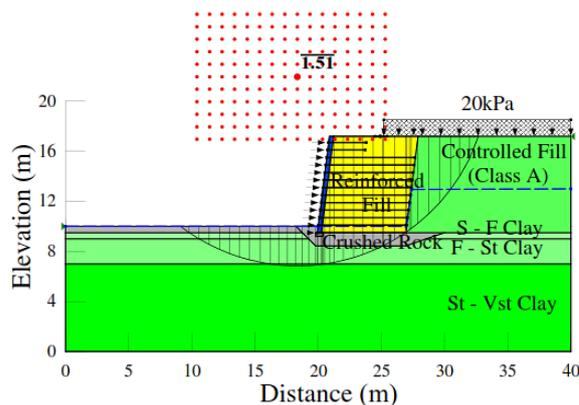
Fig. 6 FOS of geometry with ground improvement.
