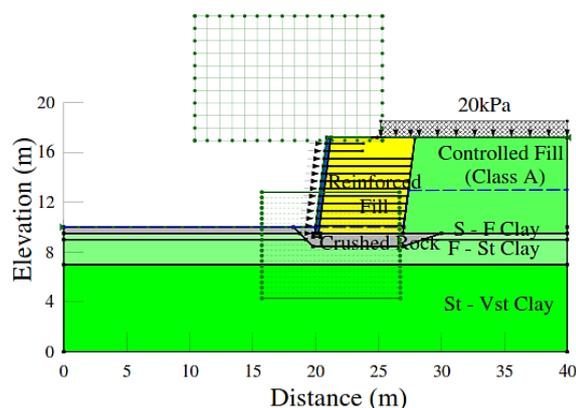
Fig. 2 Slope/W model of geometry with ground improvement.
