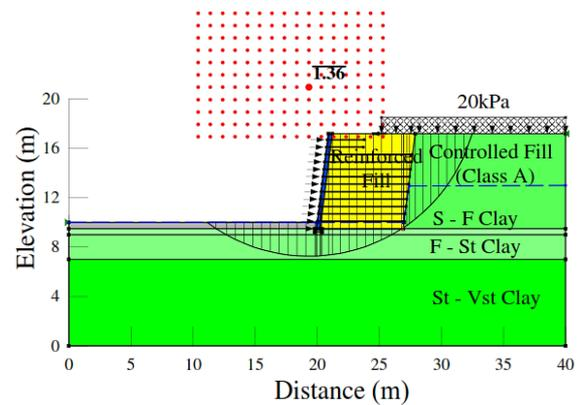
Fig. 5 FOS of geometry without ground improvement.
